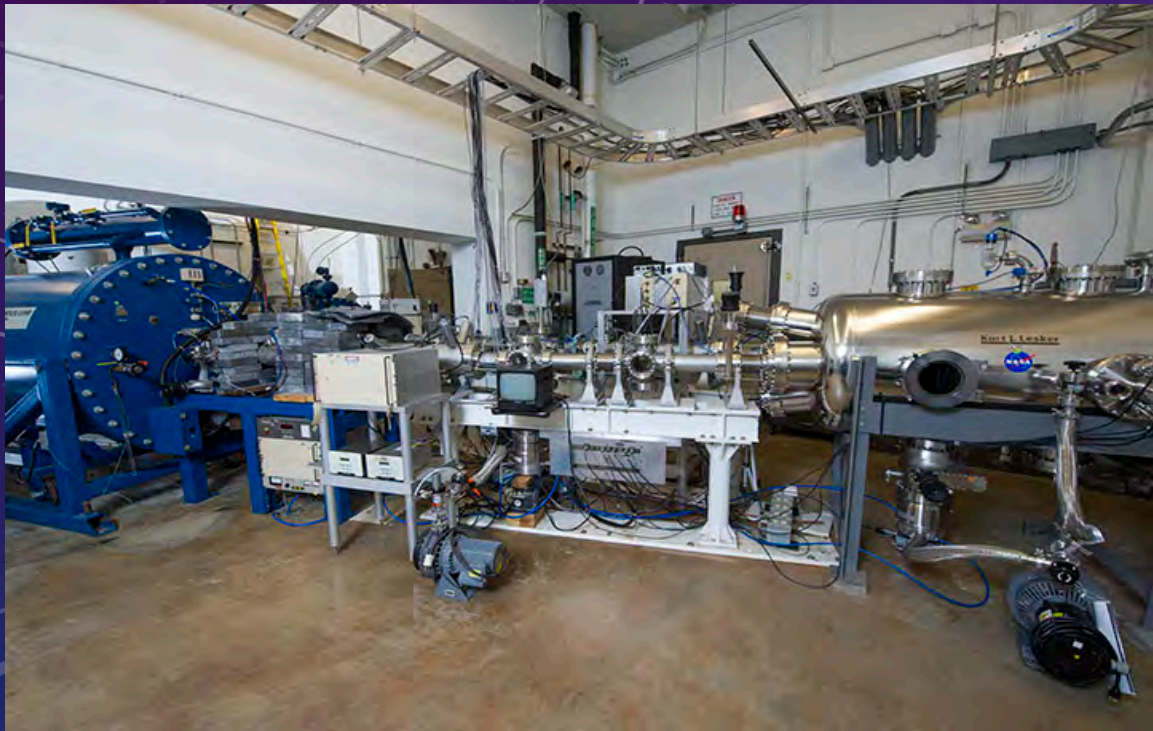
Side View of Pelletron beam line
