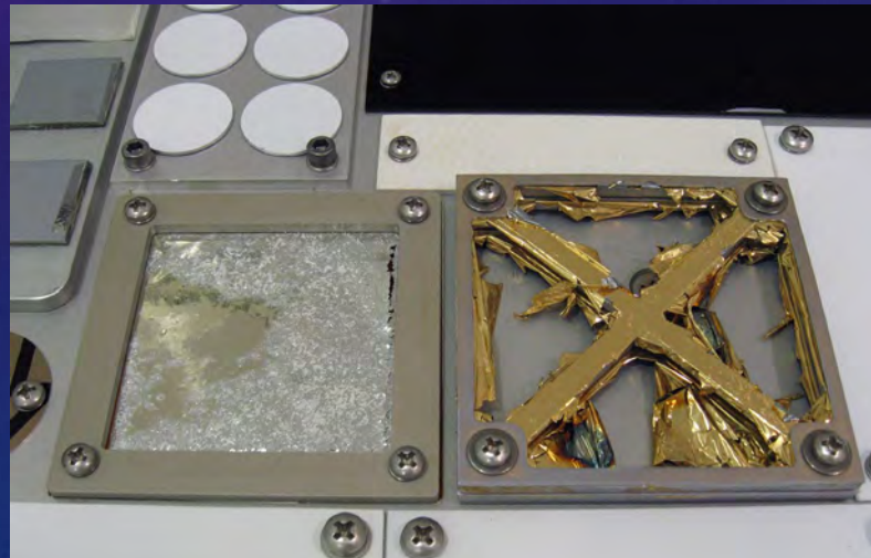
Polymer films after space exposure
